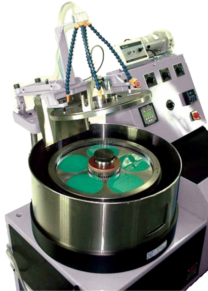
Figure 3. PR-1 double-sided lapping machine. Courtesy of P.R. Hoffman.
